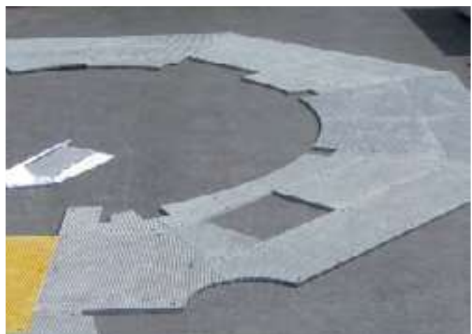
Bottom right: Quality control of GRP grating
